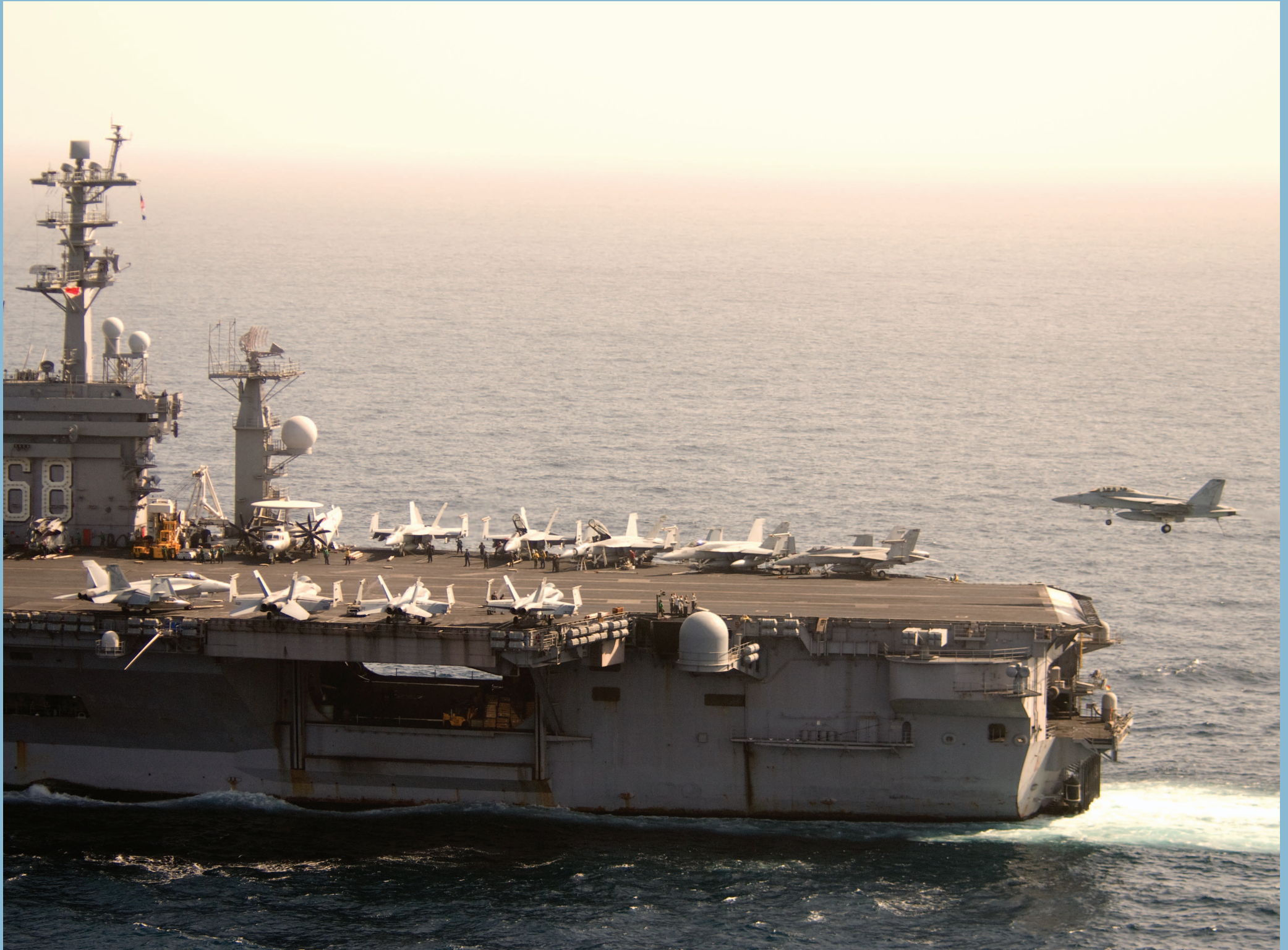
An interesting view of the Nimitz during recovery from the HS-6 helo before the RADAR ate my camera. Notice the nice, shallow angle of attack (8.1) of the Super Hornet. The F-35C is expected to have an approach AOA of 12.3, which is sure to be significantly different than the traditional sight picture from both the LSO platform and the cockpit.
