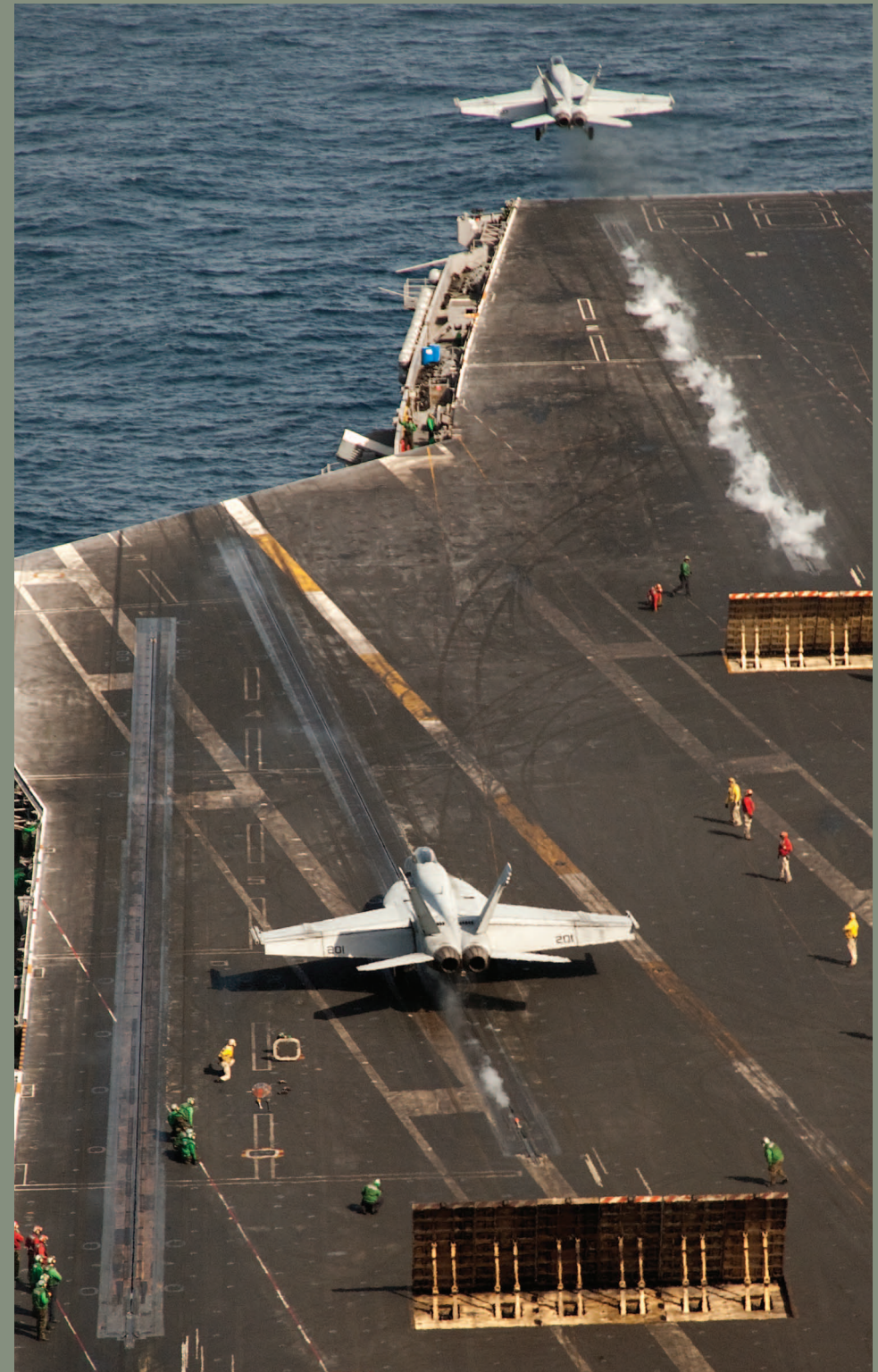
Shot from the HS-6 starboard-defense helo, this perspective shows the converging angles of the waist CATs 3 and 4. A near simultaneous or “covey” launch of 2 Super Hornets completes the first event on January 12, 2010, in the Gulf of Oman.
