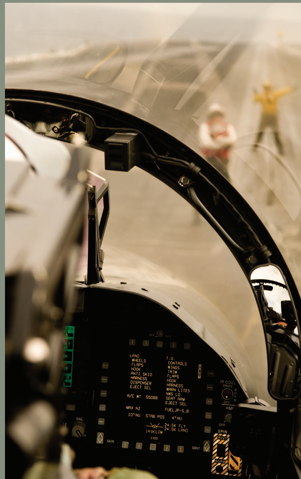
Looking over the shoulder of VFA-41's "PETA" Gendreau as he taxis our F/A-18F Rhino onto CAT 3 for a non-standard, "asym-3" high acceleration CAT shot required when a Super Hornet is configured with an asymmetric load out. Man, what a BANG! On the right multifunction display in the cockpit, you can clearly make out the pre-launch checklist page as the yellow shirt lines up the launch bar with the shuttle track.
