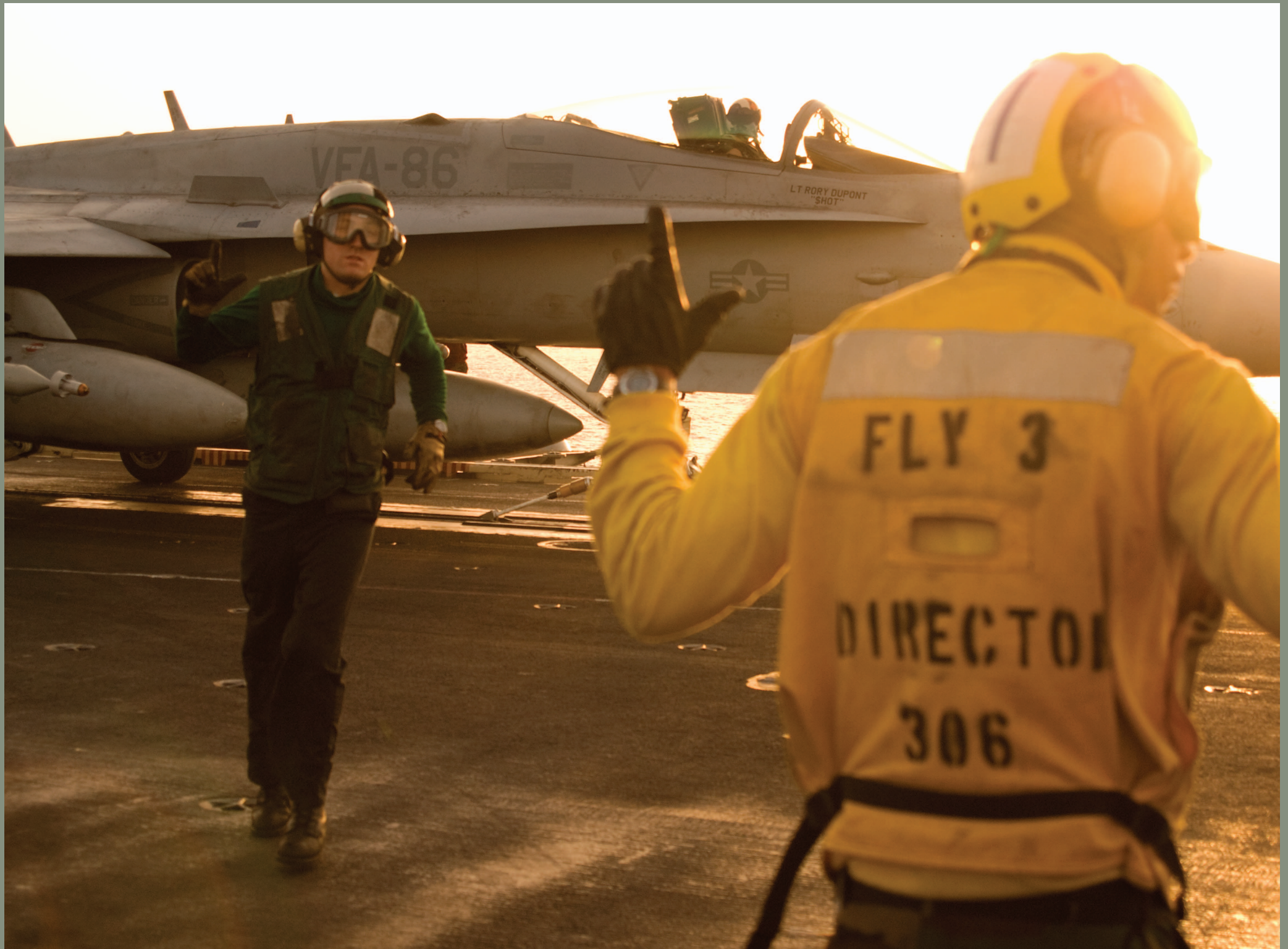
With the hold back-bar fixed and the launch bar set under shuttle tension, LCDR Eric “Frosty” Frostad flying Sidewinder #406, a legacy Hornet, is almost ready to be shot. After a salute from the pilot, thumbs up from all the checkers on the deck and finally a visual scan of the foul lines, the shooter will drop to one knee and touch the deck, settling into that tell-tale pose that means you are going for a ride.
