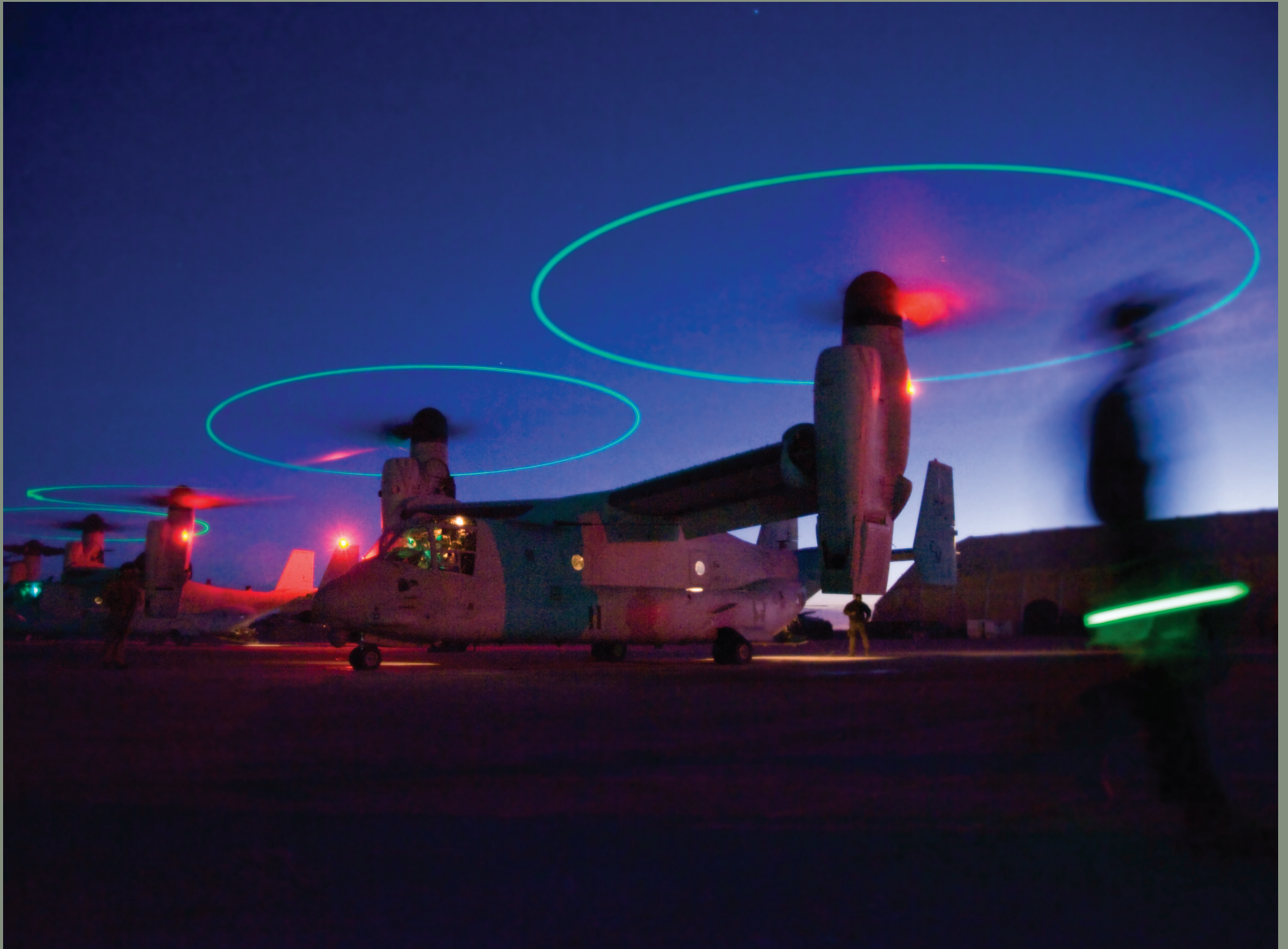
These HMM-261 Ospreys are spooling up for the day's first pre-dawn event. The green arcs are from the formation tip lights that help aircrew visualize the position of their massive rotors in the dark. From this angle, you can see there are very few windows along the side of this bird. Unless you are riding up front, there is not much to see from the air.
