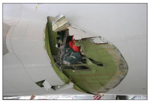
Figure 3: Extent of the fuselage rupture, after removal of further transition fairings
