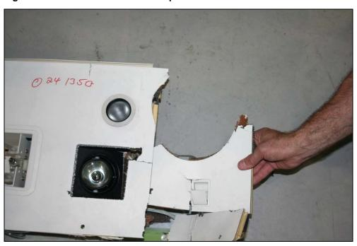
Figure 16: Panel with cut-out placed against another oxygen cylinder to illustrate the conformance in diameter
