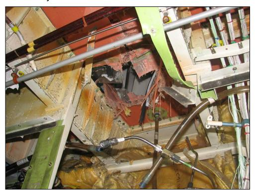
Figure 12: Door frame damage, green paint smear and rotated R2 door handle
