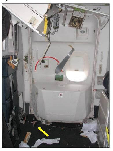
Figure 11: Hole in cabin floor – viewed from position of number-4 oxygen cylinder
