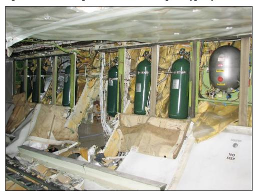
Figure 7: Fuselage rupture coincident with mounting position of the number-4 oxygen cylinder
