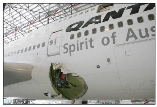
Figure 2: Fuselage rupture with protruding cargo
